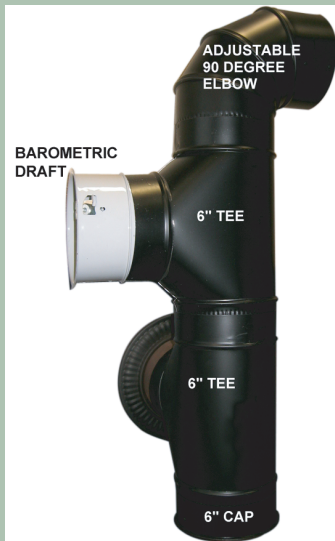
Exhaust Configuration Recommendation for exhaust with Clean Out
